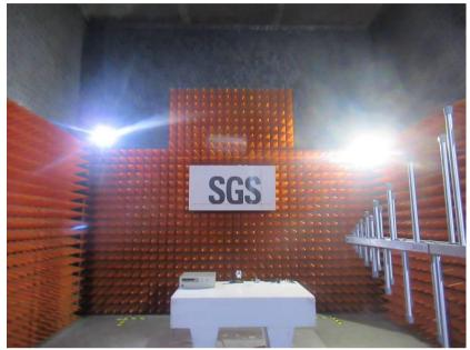
8.2 Electrostatic Discharge Test Setup
